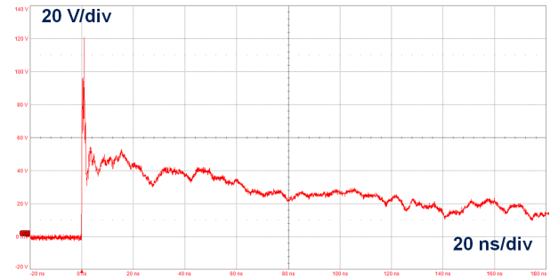
Figure 9. Response to ISO 10605 - C = 150 pF, R = 330 \Omega (+8 kV contact )
